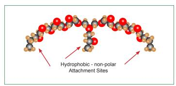
Graphic representation of Poseidon tri-block co-polymer. Additional nonpolar terminal groups provide additional sites for attachment and change the surfactant's "shape" as it sits on the particle surface.
